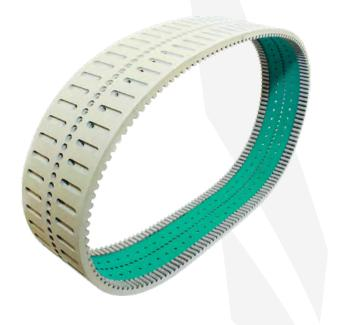
The belt, a neoprene base with a 0.125-in.-thick gray, non-marking neoprene cover, featured precision-ground teeth with slots machined into the cover, as well as holes in the slots for vacuum suction. Utilizing our advanced modification equipment, our team was able to match the original part's tooth geometry and dimension as well as spacing of the slots and holes while maintaining tolerances of ±0.01 in.
