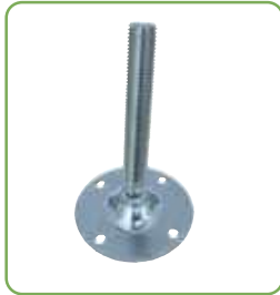
Part. R0349 - Pag. R34 Ø 123 • N. 4 holes • Stainless steel and zinc plated steel • Max. load 10000 N.
