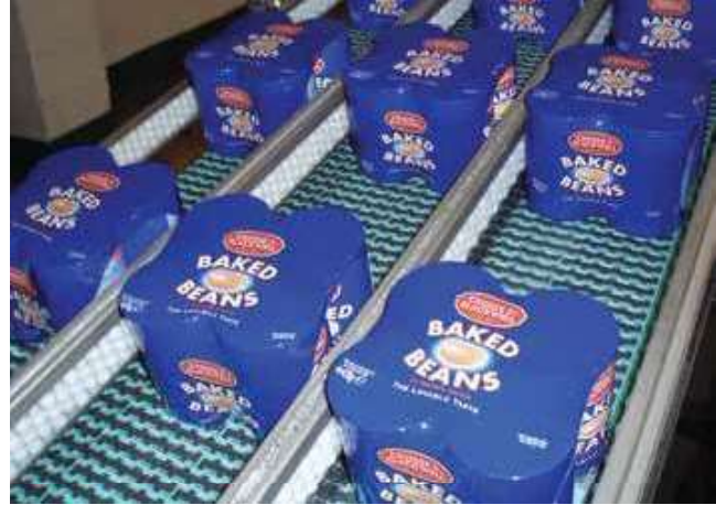
Conveyor with SGDP1505 XP Belt
