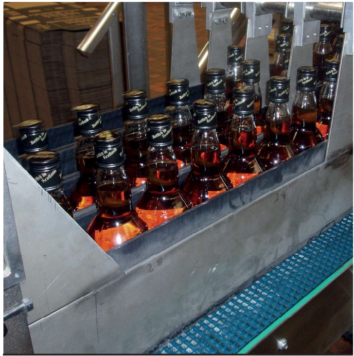
Conveyor with 500 belt.
