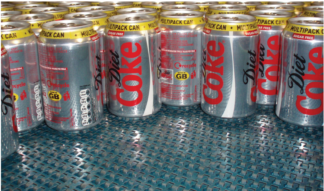
Conveyor with 500 belt.
