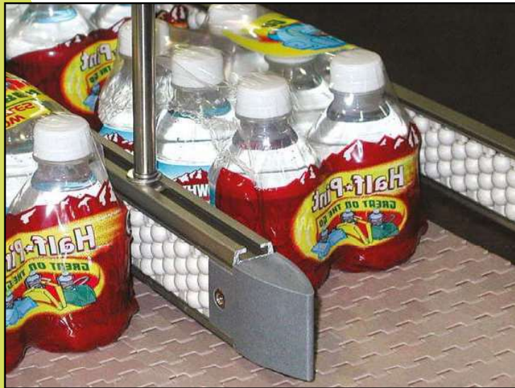
SPEEDRAIL™ ROLLER GUIDES FOR SHRINK WRAPPED PRODUCTS.
