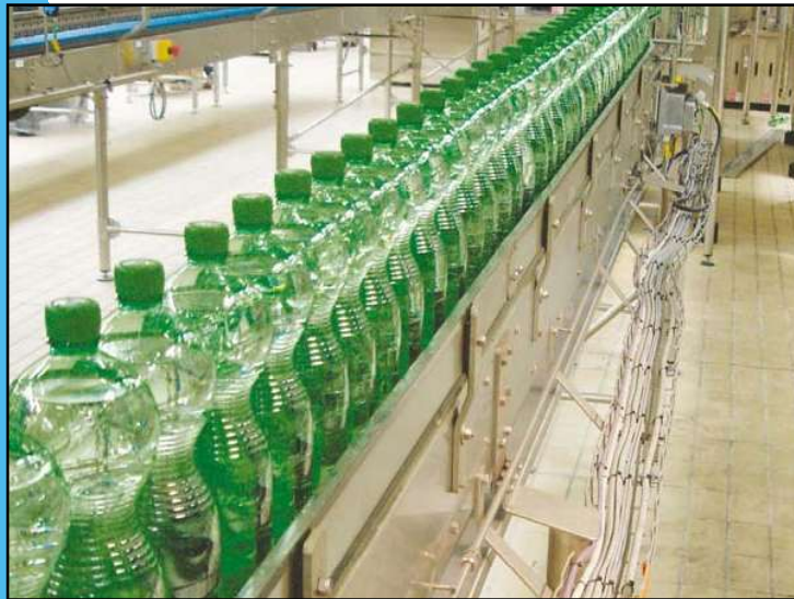
SINGLE TRACK CONVEYOR FOR PET BOTTLES.
