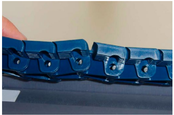
Pin in fixed position: chain can run
