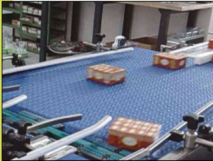
ROLLER TOP BELTS IN SORTING/POSITIONING SYSTEM.
